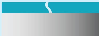
Damaged / Disrupted coating of Zinc
