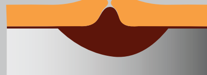
Corrosion commences due to exposure of steel
